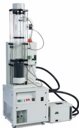
Figure 1: Experimental set-up of the Nano Spray Dryer B-90 HP with the Inert Loop B-295 and the Aspirator.
